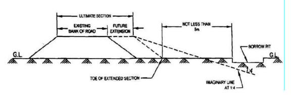
Borrow pits should not be dug continuously. Ridges of not less than 8 m width should be left at intervals not exceeding 300 m. Small drains should be cut through the ridges, if necessary, to facilitate drainage. When it becomes necessary to borrow earth from temporarily acquired cultivable lands, the depth of borrow pits should not exceed 1 m.
