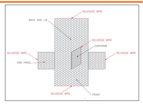
Fig 24.5 Components of Gabions
