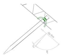
Inclination of T-steel nail
